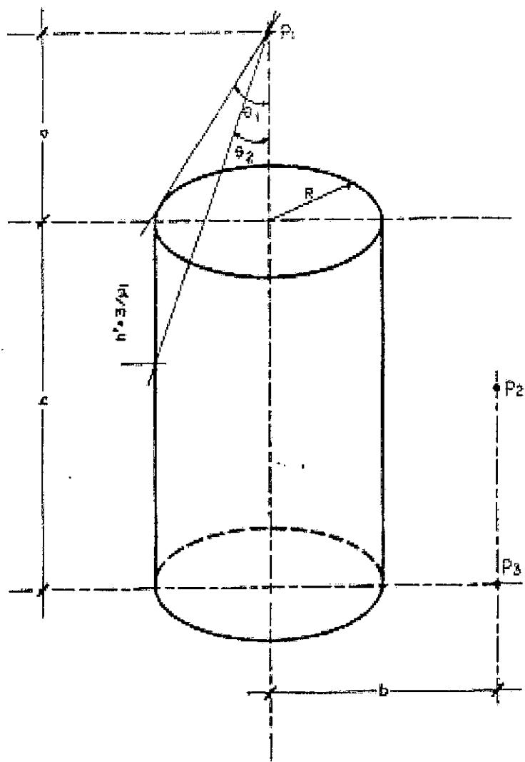
Figure 6.3. Geometry for cylinder source
